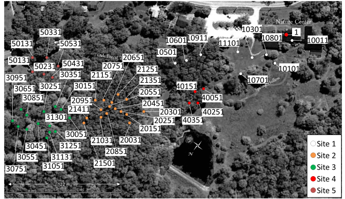
Fig. 10. An illustration of the WSN testbed deployed in a forested nature reserve at ASWP.
