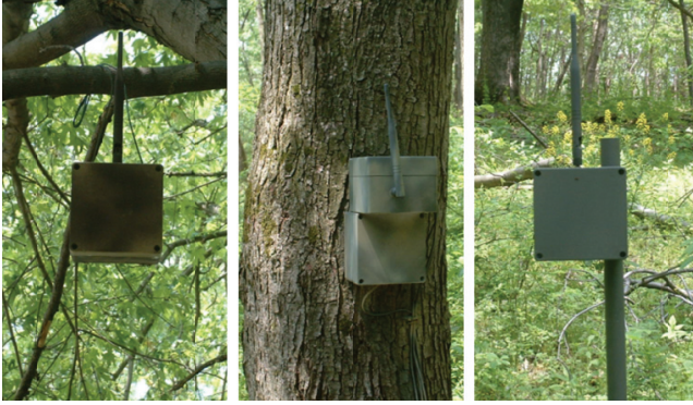
Figure 2. An illustration of deployed nodes at ASWP WSN testbed.
